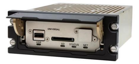
The SSDTU incorporates high speed USB and SD memory card ports for data transfers, eliminating the issues experienced with Zip disks. The SSDTU appears as a network file server to other interfaced LRUs and transfers data files between the media ports and the LRU using a high-speed Ethernet data bus connection.
